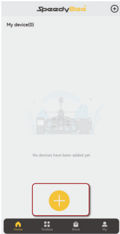
Step 1: Power on the FC. Open the SpeedyBee App, tap the "+" to connect to the FC.
